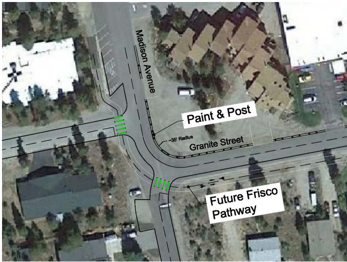
Figure 5: Concept for Stop Sign Optimization on Granite Street developed during the design charrette
